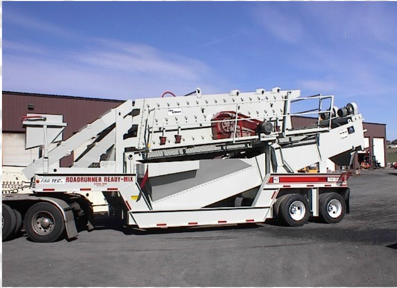
The Pro 6x16 Incline Wash plant with Twin 36" Sand Screw.
