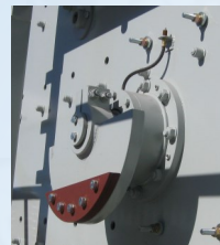
Heavy duty bearing housing with remote lube and adjustable counter-weight.
